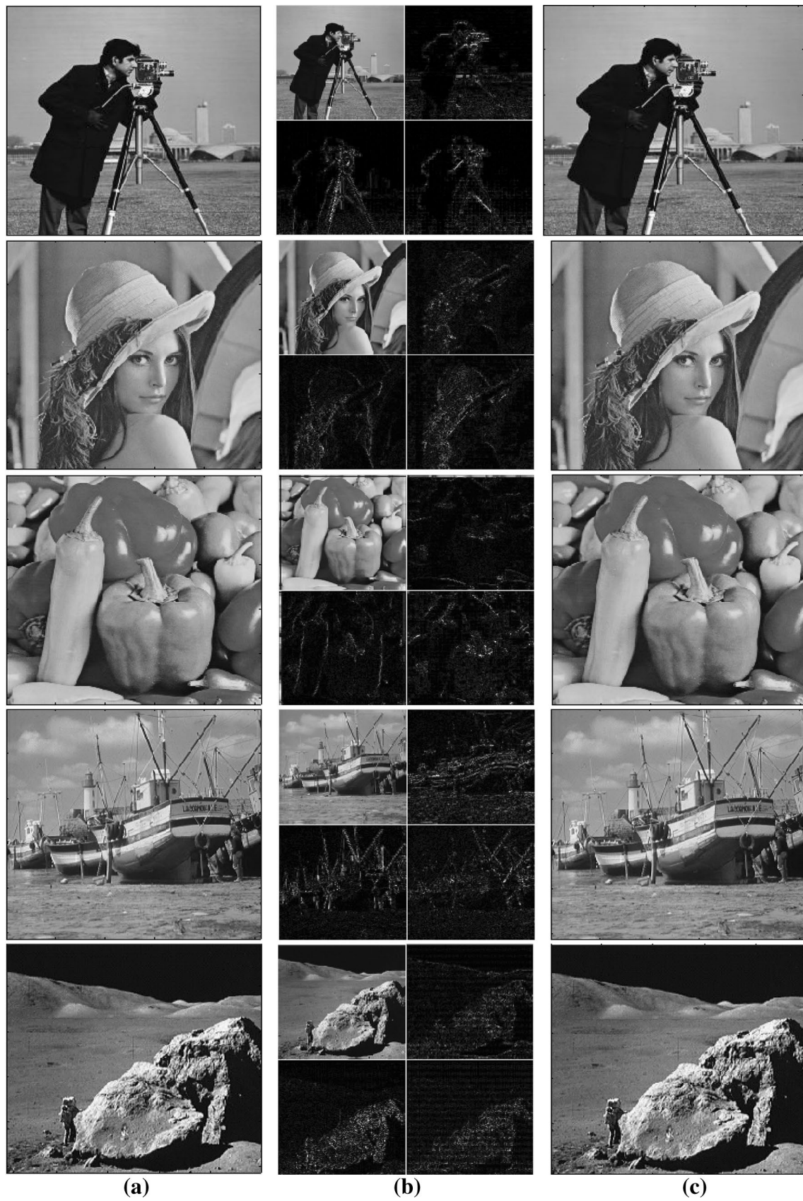
Fig. 16 a Original images; b 2D DWT decomposed images using Spartan-6, and c reconstructed images
