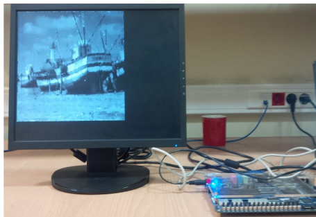
Fig. 18 Physical implementation of the system on FPGA
