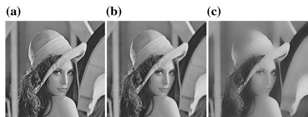
Fig. 1 Example of the impacts of BF parameters. a Original image. b d = 6 , \sigma_c = 100 and \sigma_s = 100 . c d = 50 , \sigma_c = 50 and \sigma_s = 50
