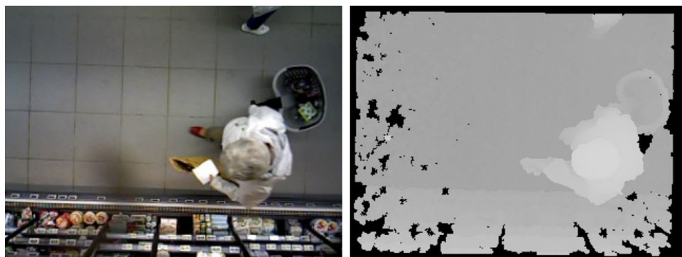
Fig. 3 The Xtion PRO-LIVE provides a color and a depth image. For the head–shoulders tracking this data makes the observation
