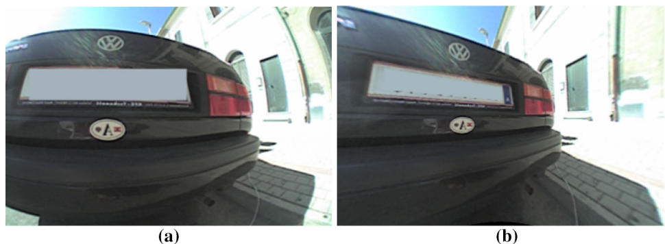
Fig. 22 Example result: a stationary car as captured from fish-eye camera, b corrected image that shows the exact angular position of the car
