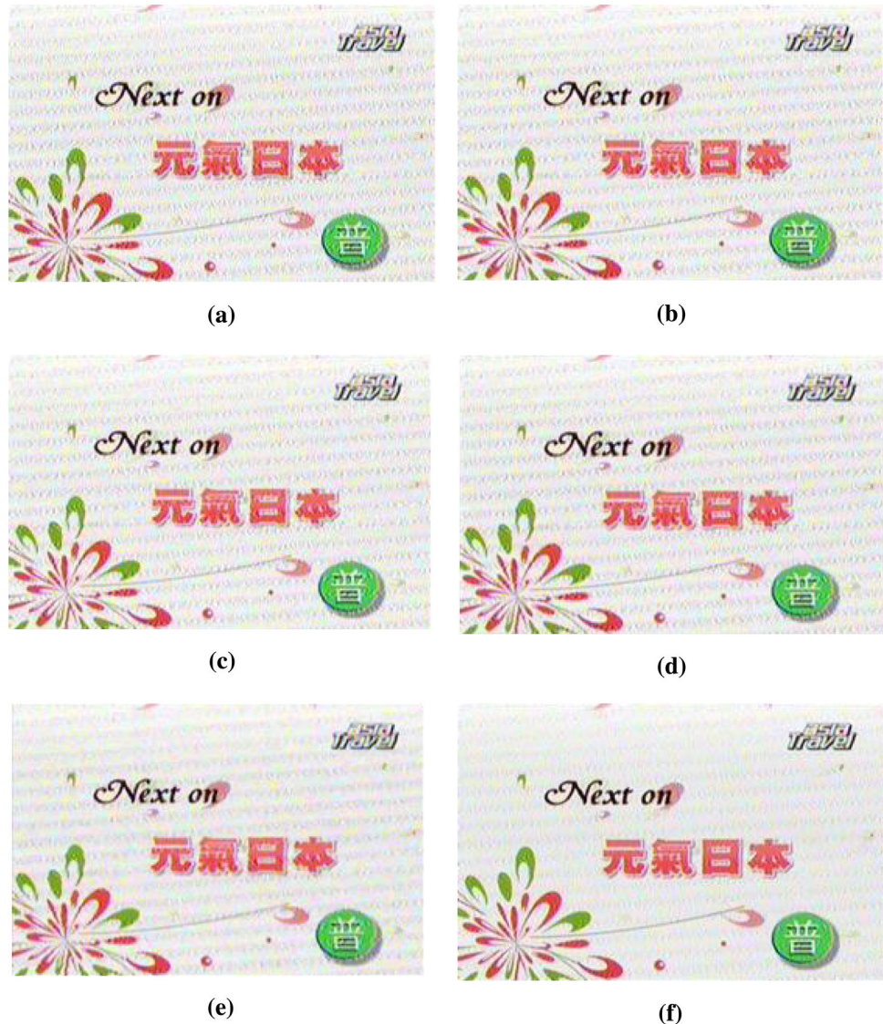
Fig. 11 a Original sampling image; b standard median filter [1]; c low-cost filter [2]; d \alpha -trimmed mean filter [8]; e STS-DDWA filter [9]; f proposed
