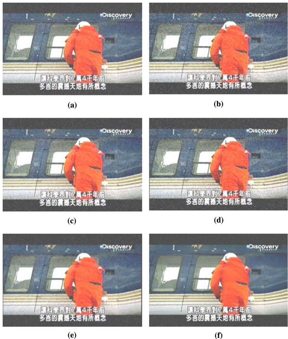
Fig. 10 a Added Gaussian noise; b standard median filter [1] (PSNR = 26.13 dB); c low-cost filter [2] (PSNR = 26.06 dB); d \alpha -trimmed mean filter [8] (PSNR = 27.67 dB); e STS-DDWA filter [9] (PSNR = 25.27 dB); f proposed (PSNR = 28.02 dB)
