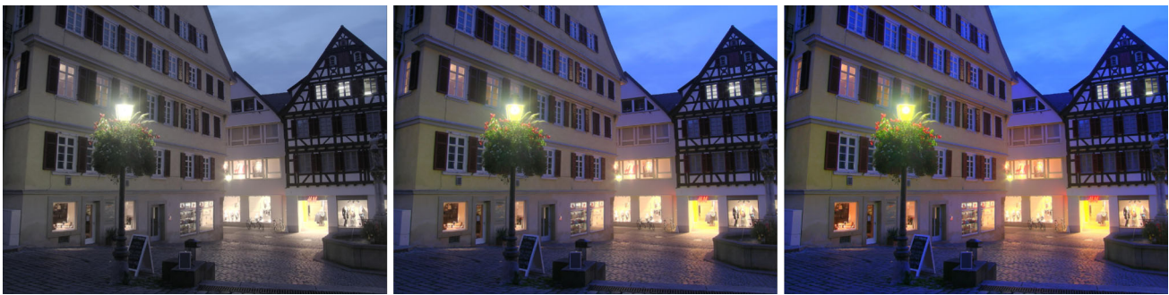
Fig. 6 The effect of changing the saturation parameter. The image on the left has the saturation parameter set to 0.5 and the image on the right to 1.5. The center image has no post tone mapping saturation adjustment (i.e. parameter set to 1.0)
