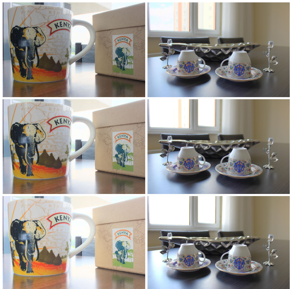
Fig. 5 The left column depicts the tone mapping results with increasing key value in each row (0.18, 0.36, and 0.72 from top to bottom ). The right column , on the other hand, depicts tone mapping results with decreasing burn-out threshold ( 10^6 , 5, and 2 from top to bottom )
