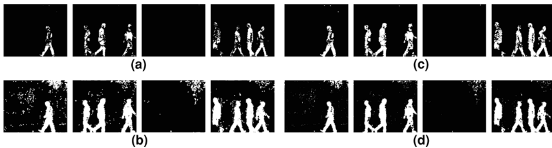
Fig. 8 Results of morphological operators on the frames shown in Fig. 4. The frames are the output of the identification circuit of Fig. (3). a Erosion, b dilation, c opening, d closing
