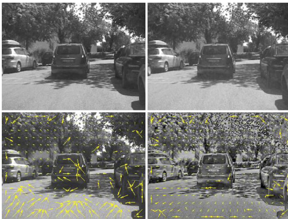
Fig. 3 Up : two adjacent frames in the test input sequence. The input images suffer for the presence of shadows both on the street and on the camera lens. Down left the motion vector field obtained without preprocessing and on the right using the proposed algorithm to pre-process the input sequence
