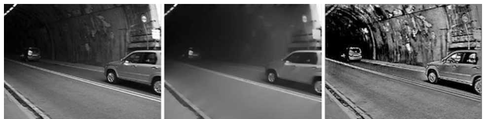
Fig. 1 From left to right: the input image acquired by the camera, the luminance estimation and the reflectance signal obtained via (9)
