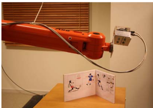
Fig. 3 The camera and the IMU are mounted onto an industrial robot. The background shows the scene that has been used in the experiments
