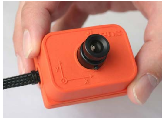
Fig. 1 A prototype of the MATRIS project, integrating a camera and an IMU in a single housing. It provides a hardware synchronized stream of video and inertial data
