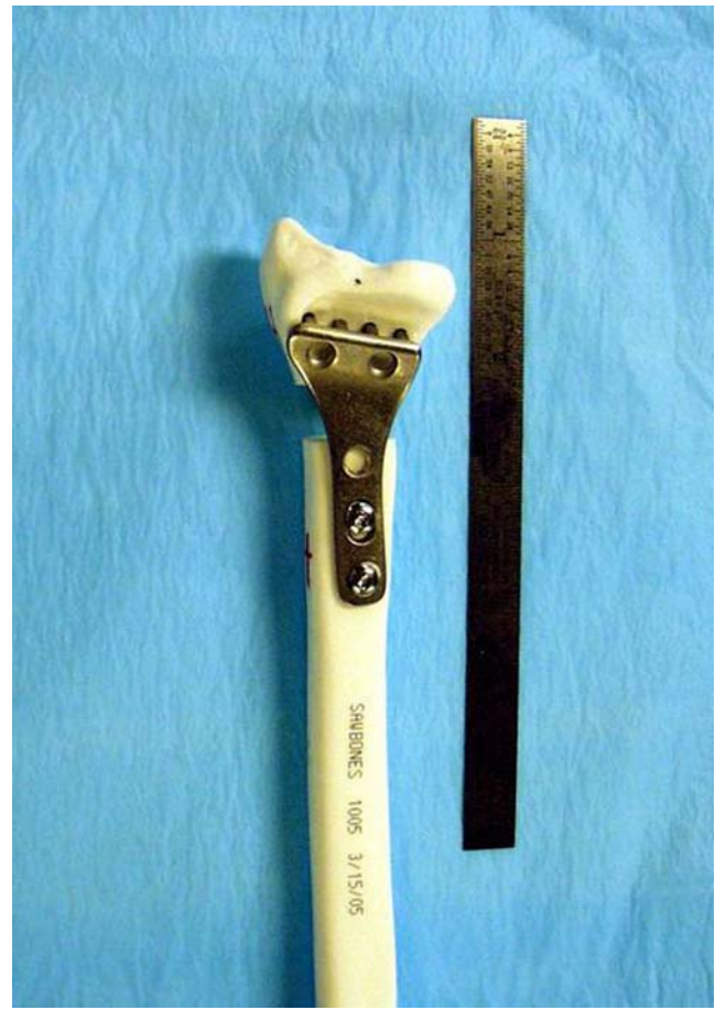
Figure 1 Specimens fixed by using three 3.5-mm bicortical proximal screws and four-fixed angle tines.
