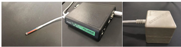
Fig. 2 Electromagnetic tracking system. Left: Microsensor; middle: processing unit; right: TX2, the electromagnetic field generator
