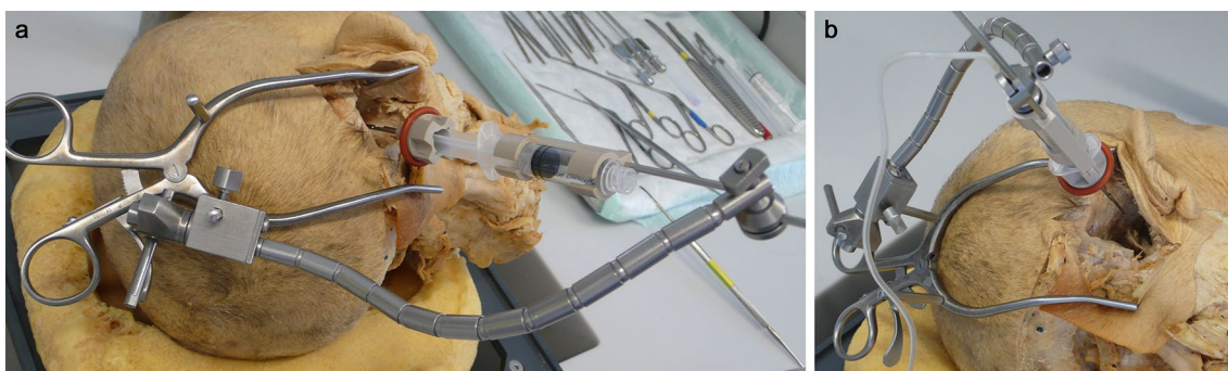
Fig. 5 Mounting of the CHD to the cadaver's head. Different positions were tested aiming the tip of the instrument deep toward the cochlea. The flexible arm provides a sufficient stable configuration
