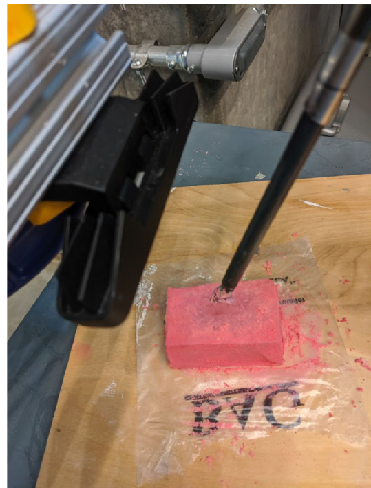
Fig. 2 Deformable phantom setup. The RGBD camera is mounted above the workspace on the left. The phantom is coated with spray paint and potato starch to improve its visibility to the depth camera
