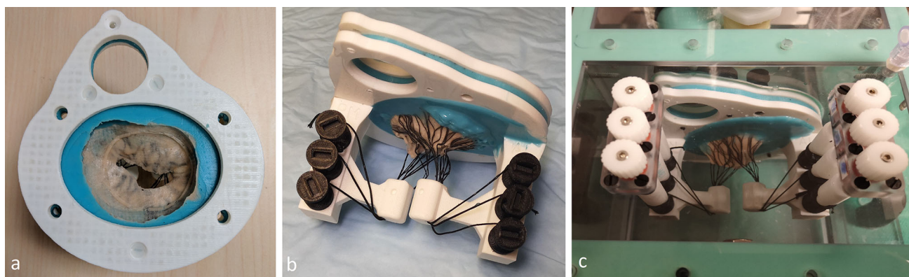
Fig. 3 a The en face view of the MV and flange; b the valve assembly with flange, papillary posts and adjustable chordae; c the valve assembly mounted in the MVS pulse duplicator. Dials on the lid of the device connect to the papillary posts so the chordae can be adjusted while the device is in operation
