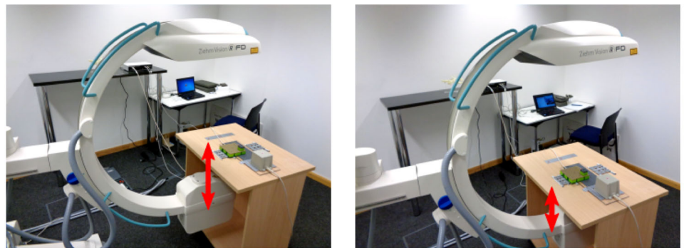
(a) x-ray source placed at short distance to setup (approx. 30 cm) (b) x-ray source at minimum realistic distance to setup (approx. 15 cm)
