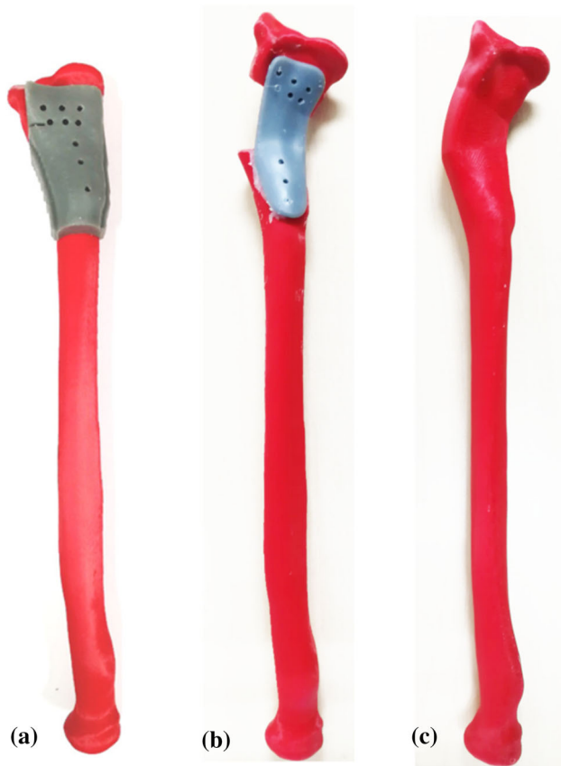
Fig. 6 3D-printed models used in the laboratory study: a affected bone models with cutting and drilling guide; b after cutting and drilling screw holes in the affected bone model, the patient-specific plate was glued to the resulting bone segments; c corrected bone model used as a reference in the laboratory study to calculate residual repositioning errors
