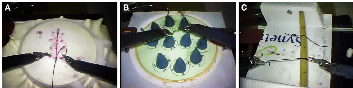
Fig. 3 Snapshots of operation tasks during robot-assisted minimally invasive surgical training. The operations are implemented using the da Vinci robot and are reported in JIGSAWS [40]: a Suturing, b Needle-passing, c Knot-tying
