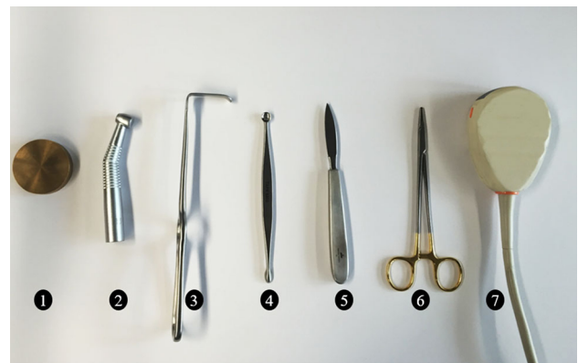
Fig. 10 Sources of distortions: 1 5 cm × 1 cm brass disk, 2 dental drill body, 3 Langenbeck hook, 4 bone curettes, 5 scalpel, 6 needle holder, 7 ultrasound probe
