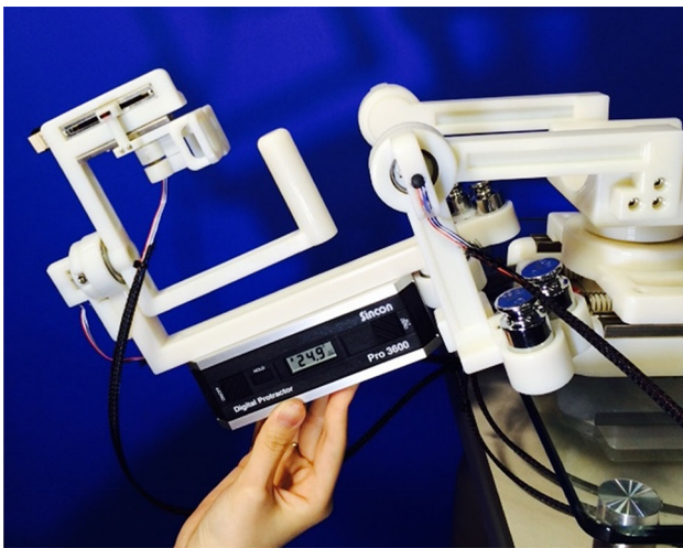
Fig. 7 The angle of joint 4 with the counterbalance masses
