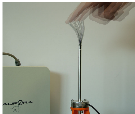
Fig. 5 Demonstration of the robot deflection under external tip load. The pressure in the muscles of the robot is kept constant, while the load on the tip is gradually increased
