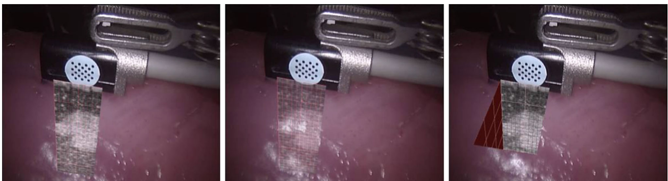
Fig. 5 Ultrasound overlay schemes: overwrite ( left ), alpha-blend ( middle ) and window ( right )
