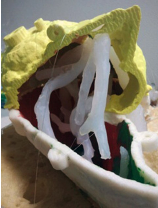
Fig. 6 Phantom liver assembly. The vessels and the lesions have been held in the correct position by means of lines. In a later step, the silicone mixture made for the parenchyma realization has been poured in the mold
