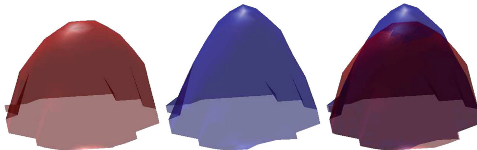
Fig. 7 Vessel cross-section intensity profile I(p_i) (left). Paraboloid intensity model \tilde{I}(p_i) (center). I and \tilde{I} overlapped (right)
