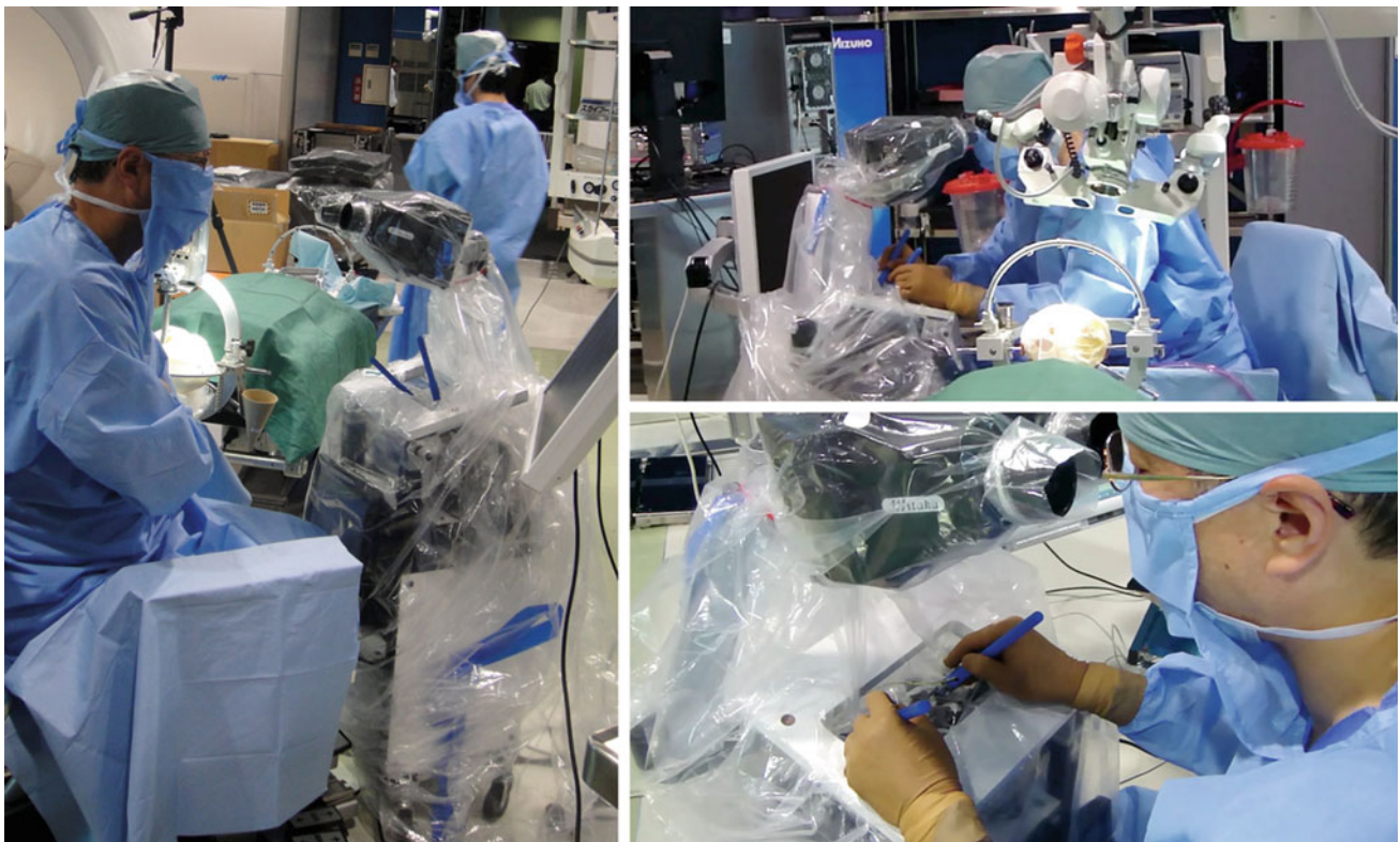
Fig. 10 The pictures show the experimental setup of the installability evaluation test. In this test, the master console was fully covered with a surgical nylon drape as it would be in actual use. The left picture shows
