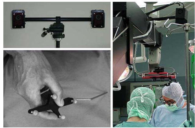
Fig. 2 Left optical tracking system and Cardio-Pointer; right optical tracking system and other equipment mounted on video robot arm
