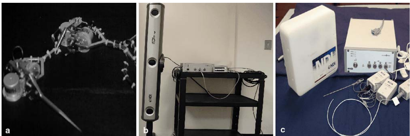
Fig. 3 Tracking systems. a Mechanical tracker (photo courtesy of Robert Galloway, Vanderbilt University), b optical tracker: Optotrak Certus (Northern Digital Inc., Waterloo, ON, Canada), c electromagnetic tracker: Aurora electromagnetic tracker (Northern Digital Inc. Waterloo, ON, Canada)
