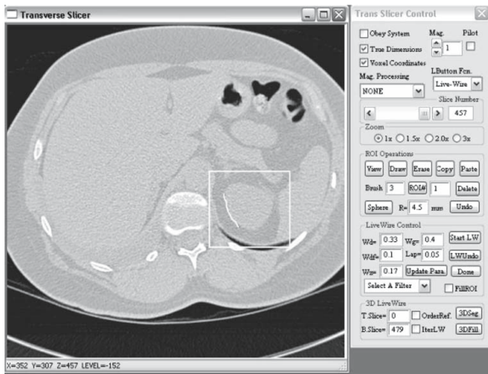
Fig. 8 Graphical user interface incorporating the proposed live wire methods. The white rectangle indicates a working rectangle specified by the user, while the enclosed white line indicates the beginning of an ROI’s definition during 2D live wire. Refer to the text for more discussion
