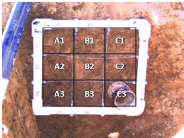
Fig. 5 Soil sampling square. Each square represents an area of 22.86 cm 2
