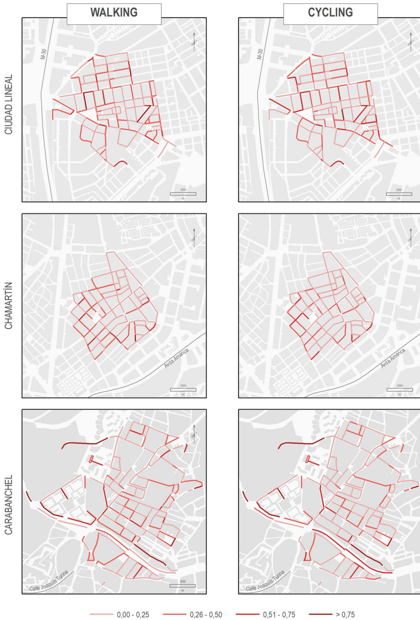
FIG. 4 Absolute differences between physical and virtual audits for walking ( left ) and cycling ( right ) total M-SPACES score.
