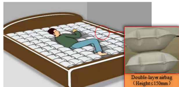
Fig. 2 Nursing bed with double-layer airbags
