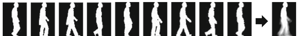
Fig. 2 Gait sequence through a series of key silhouettes, and the resulting Gait Energy Image (GEI)
