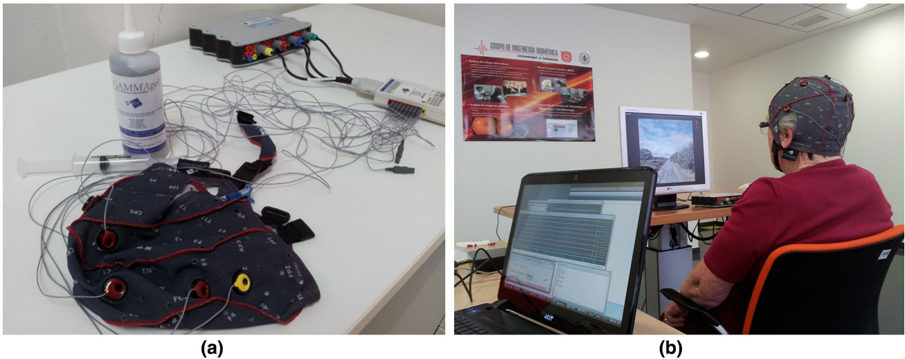
Fig. 2 a EEG recording equipment (Guger Technologies OG, Graz, Austria): the cap with eight active electrodes, the amplifier and the gel for reduce the impedance; b a real end user performing the train-
