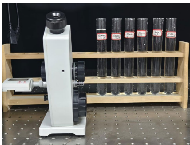
Fig. 11 Abel refractometer measurements of aqueous vitamin C solutions at concentrations of 5%, 10%, 15%, 20%, 25%, and 34% (saturated)
