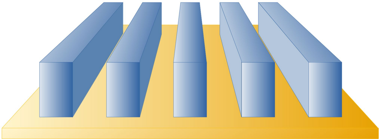
Fig. 11 The one-dimensional PhPI crystal formed by stacks of air and PMMA on a thin metallic film
