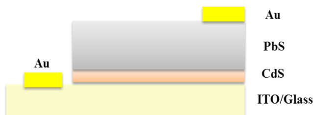
Scheme 2 ITO/CdS/PbS/Au solar cell system
