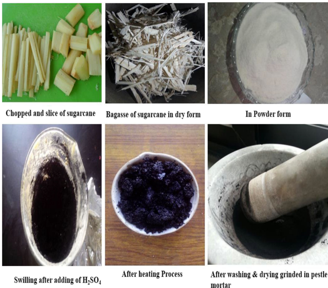
Fig. 1 Synthesis steps of carbon nanoparticles from the waste of sugarcane
