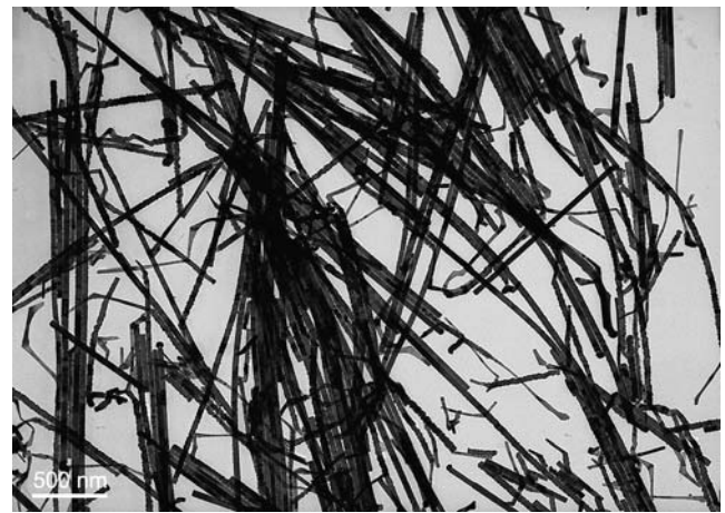
Fig. 15 TEM image of PbS NWs using gold NPs
