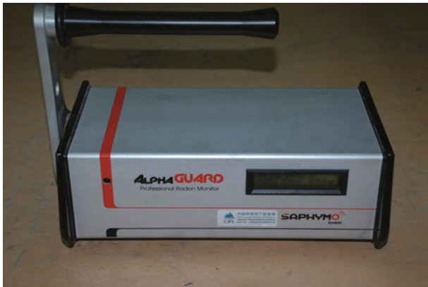
Fig. 8 Radon monitor in CJPL experiment hall.
