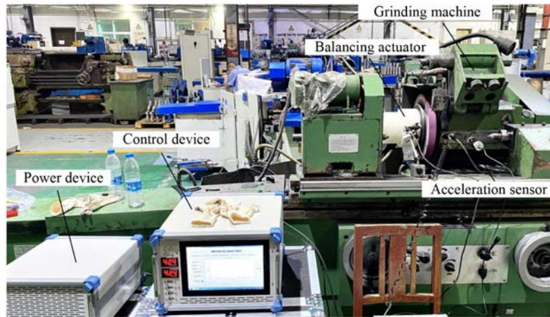
Fig. 15 A universal cylindrical grinding machine with unbalance vibration self-recovery regulation system.
