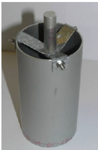
Fig. 10 Circular tube with buckling initiator. Reprinted with permission from Ref. [39] from Elsevier.
