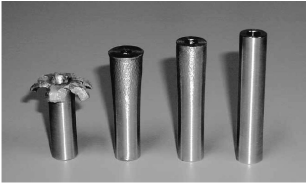
Fig. 11 Aluminum samples: Collapse mode at velocities of 361, 220, 137, and 0 m/s (from left to right). Reprinted with permission from Ref. [27] from Elsevier.
