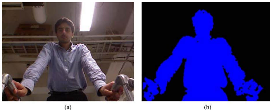
Fig. 5 (a) Color image captured by Kinect; (b) the segmented user's mask image obtained by distance slicing
