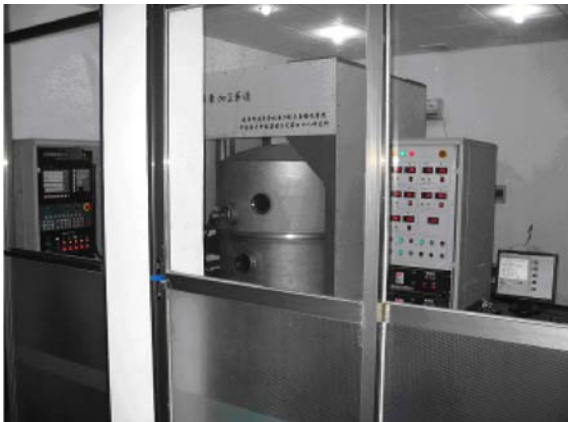
Fig. 23 IBF equipment (KDIFS-500) developed at the National University of Defense Technology
