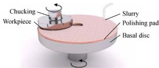
Fig. 15 Schematic diagram of CMP
