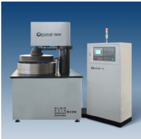
Fig. 25 Ultra-precision ball lapper Olymball-E600
