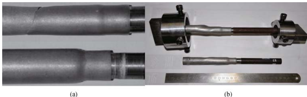
Fig. 8 Mechanical test on Al/steel joint. (a) Tensile test; (b) torsion test [19]
