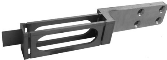
Fig. 5 Photo of the cantilever with a spring constant of 1378 N/m
