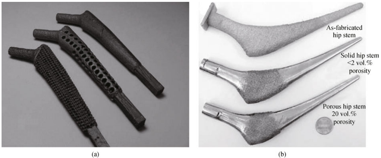
Fig. 21 (a) Hip stems with mesh, hole and solid configurations fabricated using EBM (Source: [53]); (b) functional hip stems with designed porosity (no porosity, <2 vol% porosity, and 20 vol% porosity) fabricated using LENS (Source: [101])
