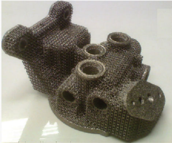
Fig. 18 Engine part with lattice structure fabricated by EBM using Ti6Al4V to reduce engine weight while enhance stiffness (Source: Arcam [124])
