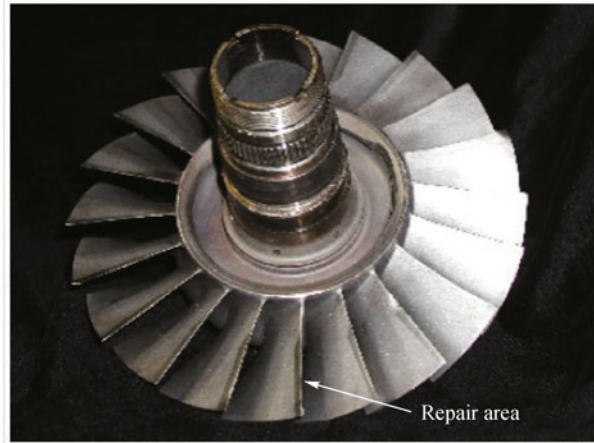
Fig. 10 Damaged blisk repaired using LENS (Source: Optomec [133])
