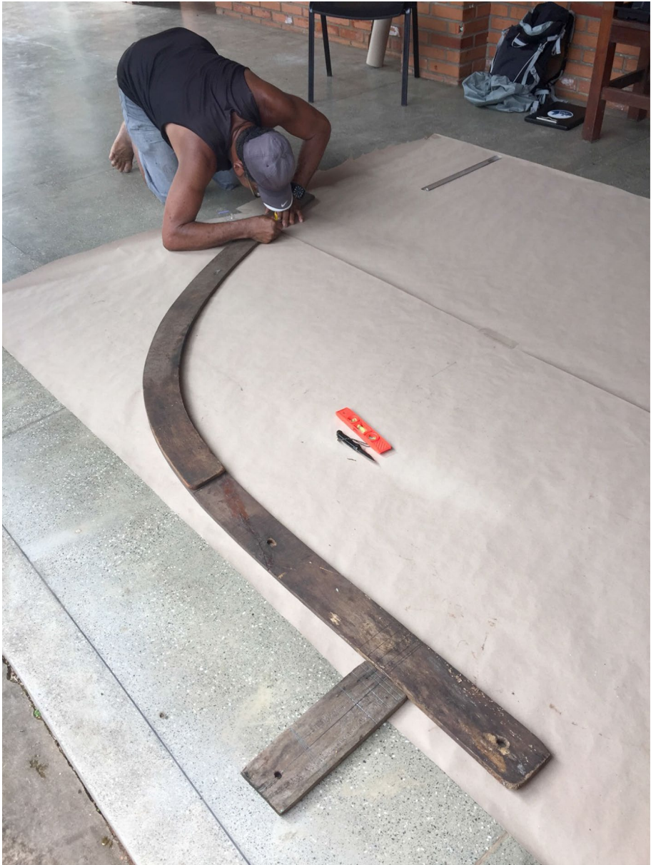
Fig. 7 Maestre Chico from Valença using his molds and graminho to demonstrate the drawing of a full size master frame. Photograph by: Rodrigo Torres
