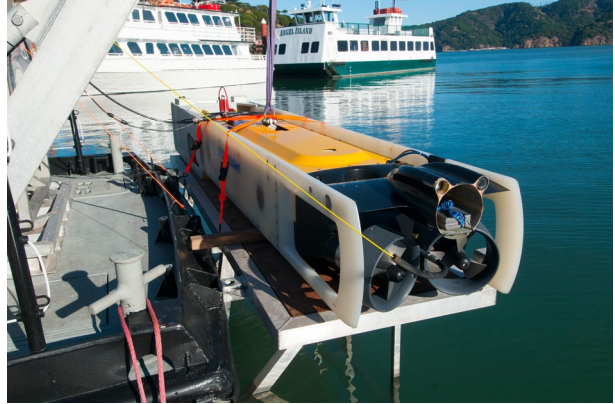
Fig. 6 R/V Eaglet 's Sabertooth AUV/ROV combination was used to survey the wrecks of SS City of Chester and SS City of Rio de Janeiro (Robert Schwemer, Office of National Marine Sanctuaries, NOAA)
