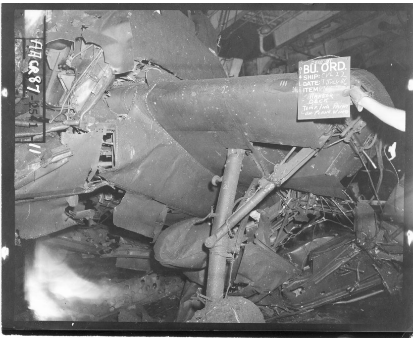
Fig. 14 Historic photo of a damaged aircraft in the forward elevator pit following the Able test. National Archives
