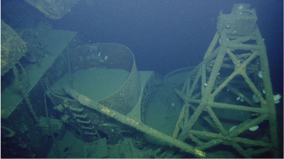
Fig. 13 ROV image of “Christmas tree” blast gauge tower still in position in the forward 40 mm gun tub at the bow. Image courtesy of Ocean Exploration Trust
