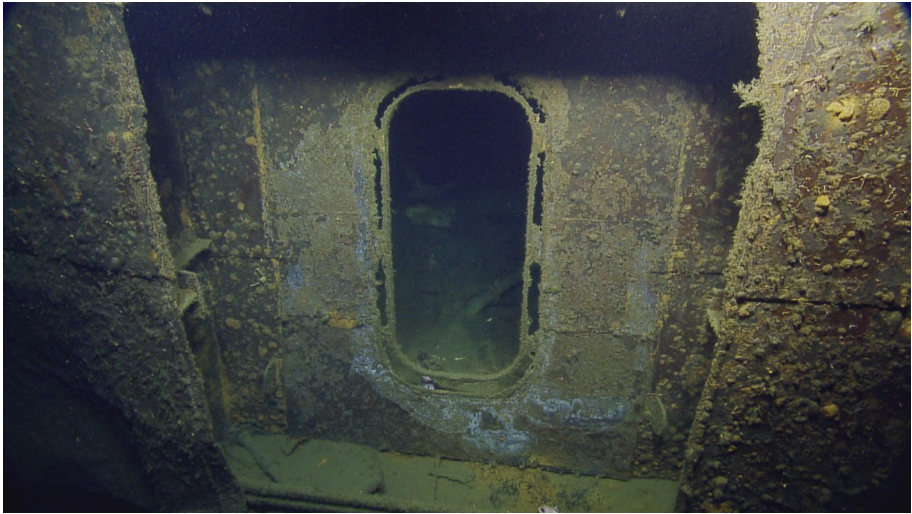
Fig. 17 ROV image of an access door cut through a hatch on the starboard side of Independence , above the torpedo blister near frame 130. Image courtesy of Ocean Exploration Trust
